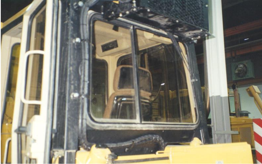
Hose routing down back of cab.
