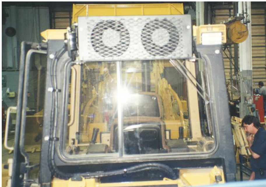
Condenser assembly viewed from back of machine.
