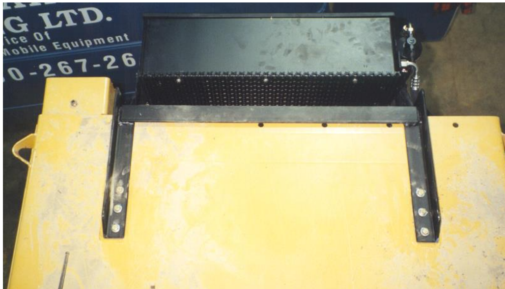
Condenser mounted with brackets in place.
