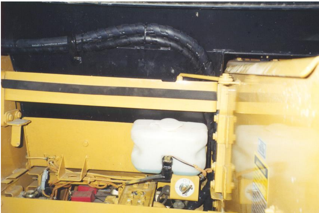
Hose routing across back of cab and down underneath.
